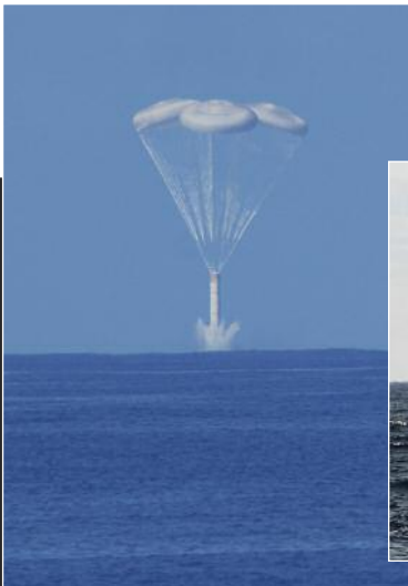
After launch, Solid Rocket Boosters separate from the Space Shuttle and are recovered in the Atlantic Ocean, close to Florida's East Coast.
