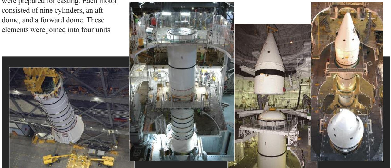
Inside the Vehicle Assembly Building, technicians complete the process of stacking the Solid Rocket Booster components.
