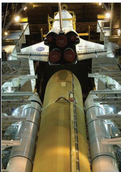
The Orbiter is then mated with the External Tank and the Solid Rocket Booster.
