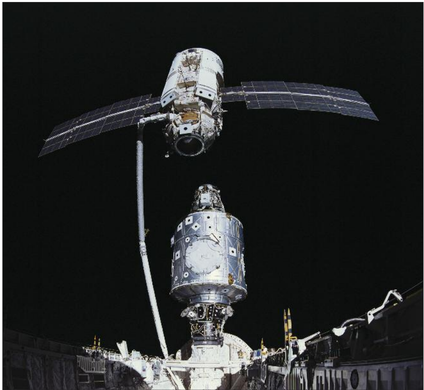
STS-88 (1998) Endeavour's Shuttle Robotic Arm grapples the Russian Module Zarya for berthing onto the International Space Station (ISS) Node 1, thus beginning the assembly sequence for the ISS.
