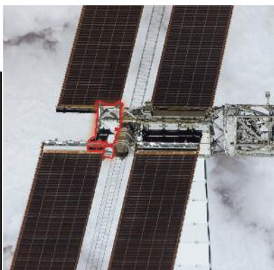
Endeavour (STS-118) delivered the S5 truss segment.
