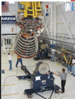
Inside the Orbiter Processing Facility, technicians process the Space Shuttle Main Engine and install it into the Orbiter.
