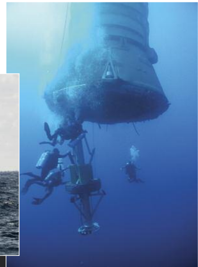
After launch, Solid Rocket Boosters separate from the Space Shuttle and are recovered in the Atlantic Ocean, close to Florida's East Coast.
