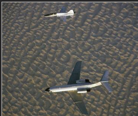
Two aircraft stationed at Ellington Air Force Base for Johnson Space Center are captured during a training and familiarization flight over White Sands, New Mexico. The Gulfstream aircraft (bottom) is NASA's Shuttle Training Aircraft and the T-38 jet serves as a chase plane.
