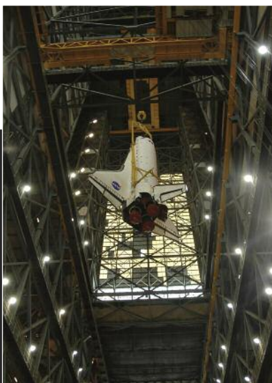
The Orbiter is then mated with the External Tank and the Solid Rocket Booster.
