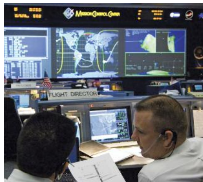
The Mission Control Center front room houses the capsule communicator, flight director and deputy, and leads for all major systems such as avionics, life support, communication systems, guidance and navigation, extravehicular activity lead and robotic arm, propulsion and other expendables, flight surgeon, and public affairs officer. These views show the extensive support and consoles. Left photo: At the front of the operations center are three screens. The clocks on the left include Greenwich time, mission elapsed time, and current shuttle commands. A map of the world with the shuttle position-current orbit is in the center. The right screen shows shuttle attitude. Center photo: Flight Director Norman Knight (right) speaks with one of the leads at the support console. Right photo: Each console in the operations center has data related to the lead's position; e.g., the life support position would have the data related to Orbiter air, water, and temperature readings and the support hardware functions.
