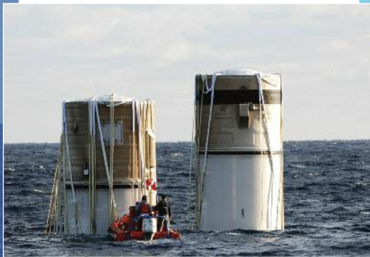
After launch, Solid Rocket Boosters separate from the Space Shuttle and are recovered in the Atlantic Ocean, close to Florida's East Coast.
